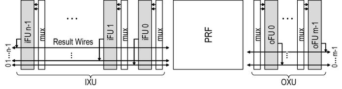
Figure 5: Bit-slice of bypass network.
