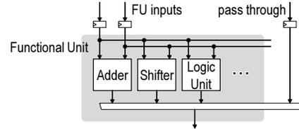
Figure 6: Functional Unit in IXU
