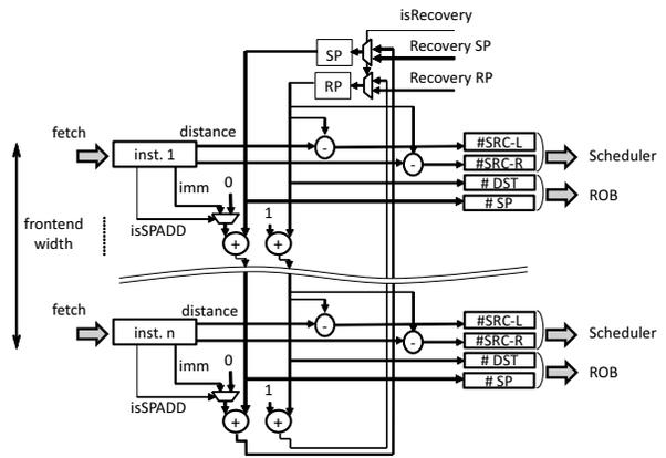
Fig. 3. The mechanism of operand determination in the front-end pipeline
