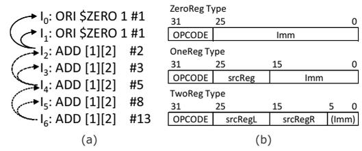
Fig. 1. Example of STRAIGHT code and bit-field formats
