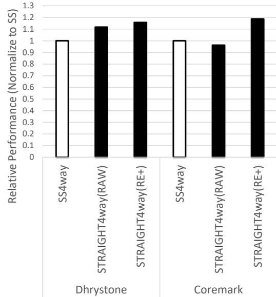
Fig. 11. Performance comparison of STRAIGHT and SS (4way)
