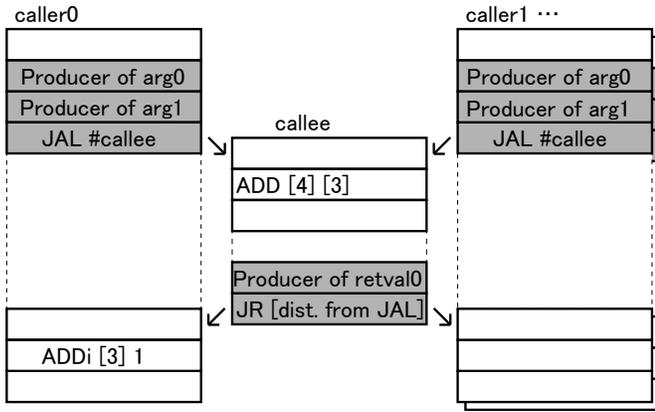
Fig. 6. Flows of Basic Blocks in Calling
